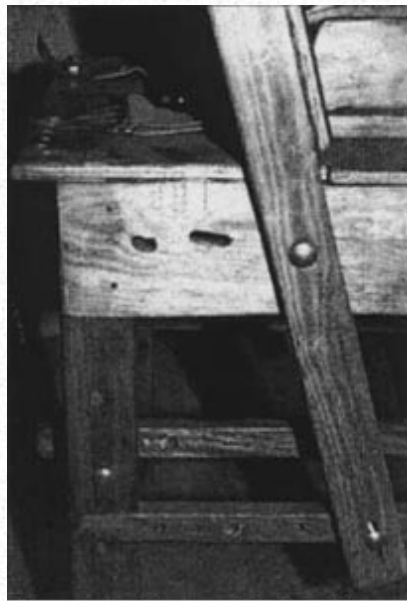
The angle of the seat back and the depth of the seat are adjustable, with bolts that pass through holes in the side boards and the bottom rungs of the chair.
