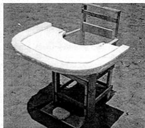
Participants made a child's seat from scraps of wood and foam plastic. They put a raised border on the table to help keep toys from falling off.
