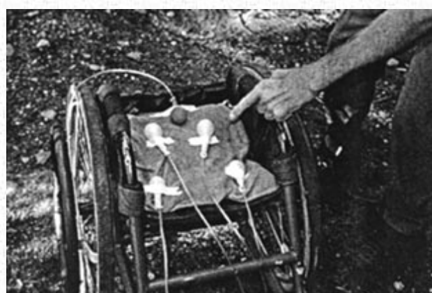
Balloons of the pressure tester are positioned on the wheelchair seat. They can be held in place with strips of sticky tape.
